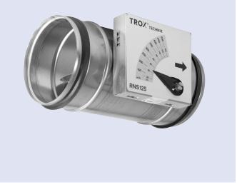
TROX Type RNS and RN volume flow controllers are mechanical system-powered controllers and were developed for the control of flow rates in constant volume systems. The controllers are suited for both supply air and extract air.
