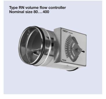
Aerodynamic forces from air flow create a closing force on the damper blade. A self inflating bellows amplifies this force, acting simultaneously as an oscillation damper. This closing force is counteracted by a leaf spring that unrolls over a cam plate. The cam plate is designed such that as the pressure differential changes, the damper blade adjusts to keep a constant flow rate within close tolerances.
