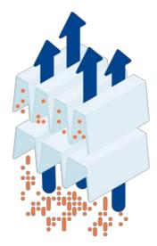
TROX's two-stage, high-performance filter system cleans the air and demonstrably filters over 99.95% of all aerosols. Aerosols which may also be contaminated with a virus. A highly efficient H13 HEPA filter is used for this purpose, HEPA filters being widely used for air cleaning in operating theatre applications.
