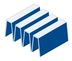
In contrast to conventional flat filter plates, the filter panels in the TROX AIR PURIFIER are concertinaed. As a result, the unit has a total filter area of  $47~\text{m}^2$ .
